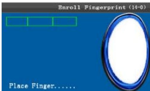
Press finger according to device's prompt. Press the finger three times in the proper way.
