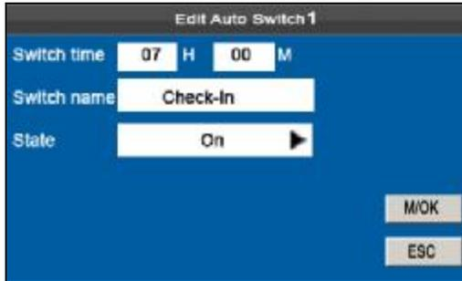
Press ▲/▼ to switch among the entry boxes. Enter the switch time using the numeric keypad and the switch name using the T9 input method. Press ◀/▶ to choose a state. After the setting is complete, press **M/OK** to save and go back to the previous interface. Press **ESC** to cancel the setting and go back to the previous interface.
