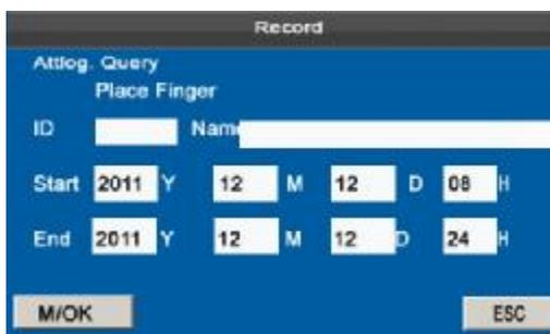
1. Two ways for entering the query conditions: 1) Press the enrolled finger, and the user ID and the name corresponding to the fingerprint will be automatically displayed. 2) Enter the desired employee information at **ID** and **Name**.
