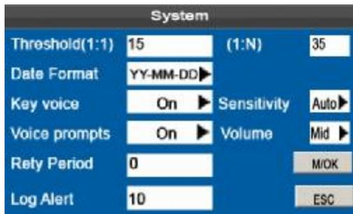
**Threshold (1:1):** This option is used to set the extent of matching between an input ID/fingerprint and that stored in templates in the ID and fingerprint identification mode.
