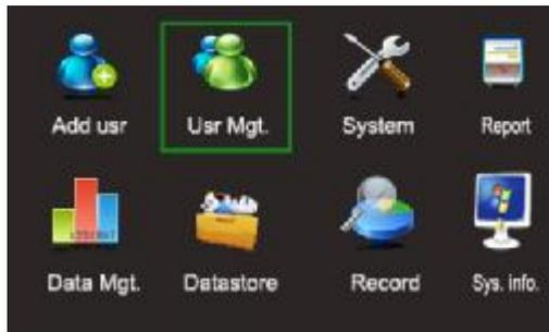
Press **◀▶** to select **User Mgt.** or press **2** to display the **User Mgt.** interface.
