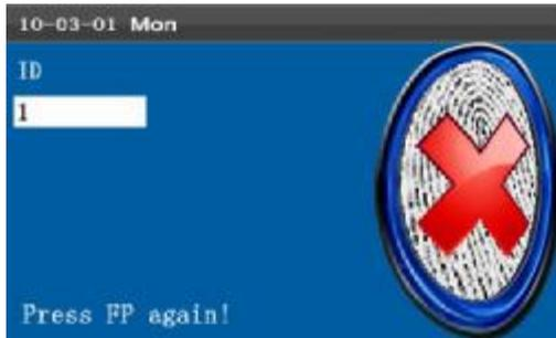
Employee can try another 2 times by default. The repeated times can be set in [4.1 System Setting](#) option. If it fails after 2 times, return Step 1 for second operation.
