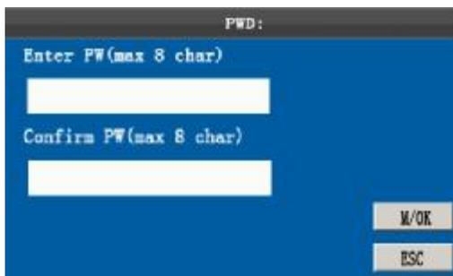
Input password (1~8) according to device's prompt, and press **M/OK** to verify it. Then press **M/OK** save it or press **ESC** to exit without saving it.
