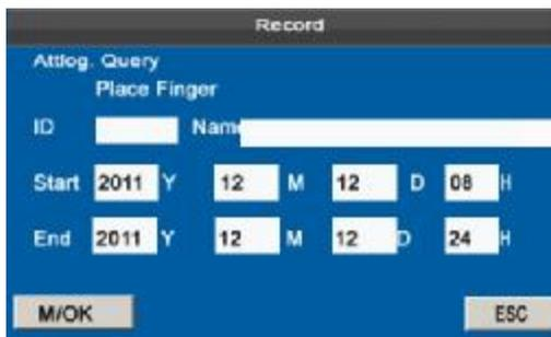
1. Two ways for entering the query conditions: 1) Press the enrolled finger, and the user ID and the name corresponding
