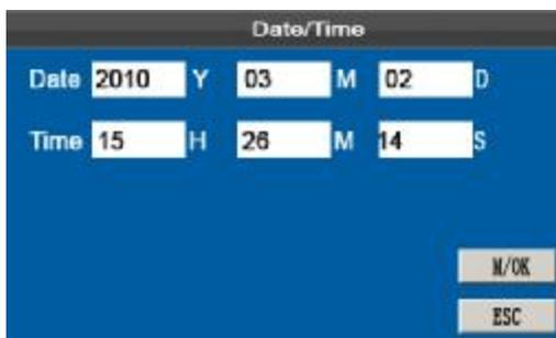
Press ▲/▼ to switch among several entry boxes. Enter the desired value by using the keypad. If you enter a time value in the wrong format, the system will display a prompt “Wrong time!” and you need to re-enter a correct value. After finishing the settings, you can press **M/OK** to save your settings and return to the previous interface, or press **ESC** to cancel your settings and return to the previous interface.
